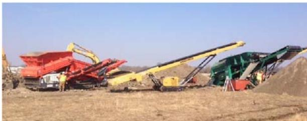
Above: Excavated soil is dumped into a hopper (at left) which is then conveyed to various-sized sifting units. Each unit expels material that won't fit through its operation into a hopper for further investigation. Below: "Fines" are the soil that filters through this sifter, smaller than 1/4". Lime is added to the clay soil to aid sifting.
