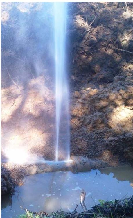
A line break in the 1940s-era cast iron water main spewed water several feet into the air.
