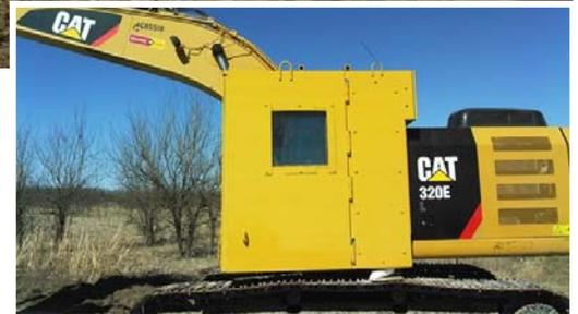
Clockwise from top left: Recovered BLU-26 cluster bombs being prepared for controlled detonation. An armored excavator moves soil in the 2700 Area. The excavator was specifically outfitted with steel plating to protect the operator. A bulldozer has been armored with heavy glass to protect its operator.
